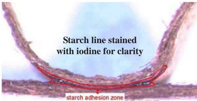
GRADE: 35-26m-35 C-Flute BEFORE ISO-BAR INSTALLATION
